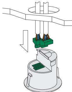
**EN** Wire in plug/s, using wiring diagram on page 3 as a guide. Connect the plug/s to the detector.
