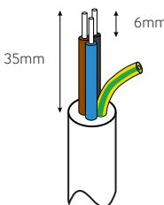
**EN** Strip the wires as shown opposite. Presence detector does not require earth conductor.
